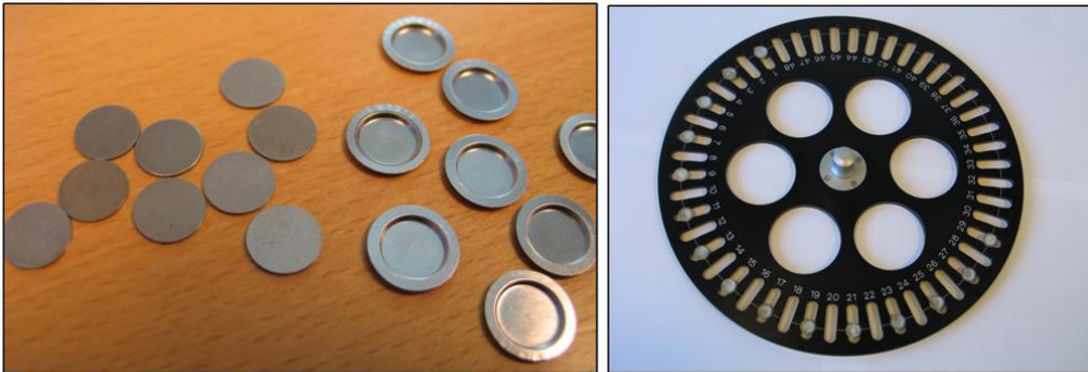
Figure 2.1: Sample discs and cups (planchettes) are shown on the left. On the right a sample carousel (sometimes referred to as “turntable”) is shown.
