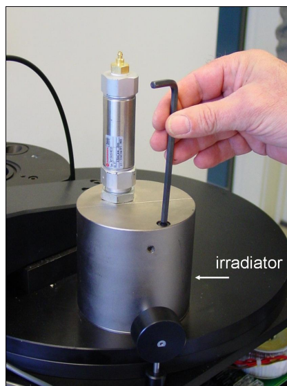
Figure 4.13: Removing the irradiator.
